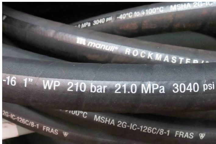
Figure 5: Hydraulic hose indicating the maximum working pressure
