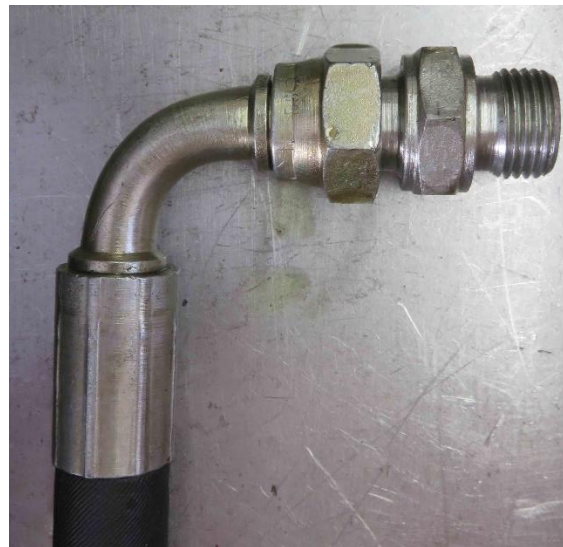
Figure 6: hose with a crimped connector and double male adaptor
