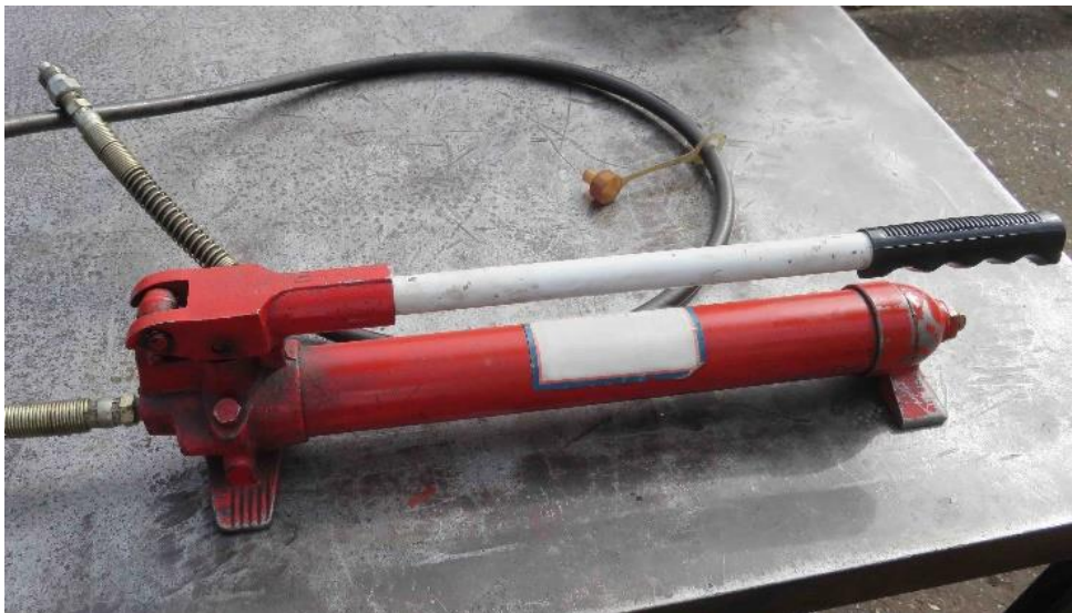
Figure 9: Example of a hand-operated external power pump (without built-in pressure gauge)
