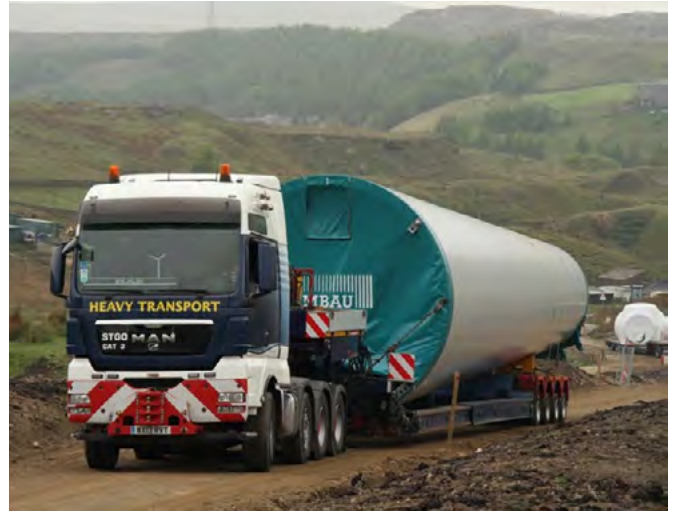
Figure 29: Typical WTG tower base section transport
