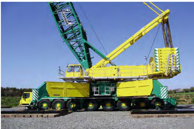
Figure 3. 750 ton lattice boom crane on outriggers with an undercarriage on tyres.
