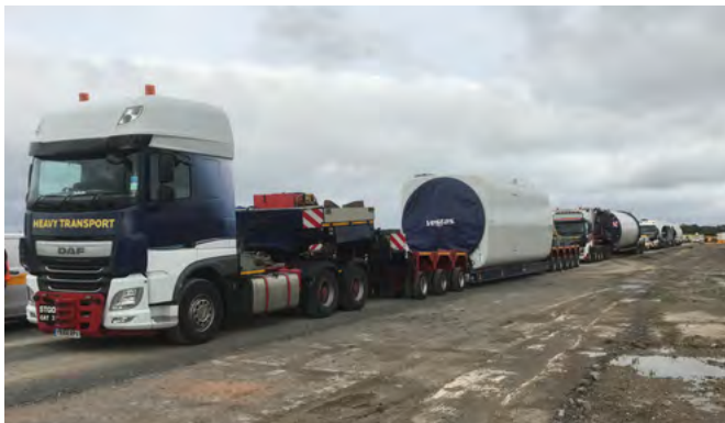
Figure 25: Typical wind turbine transport convoy
