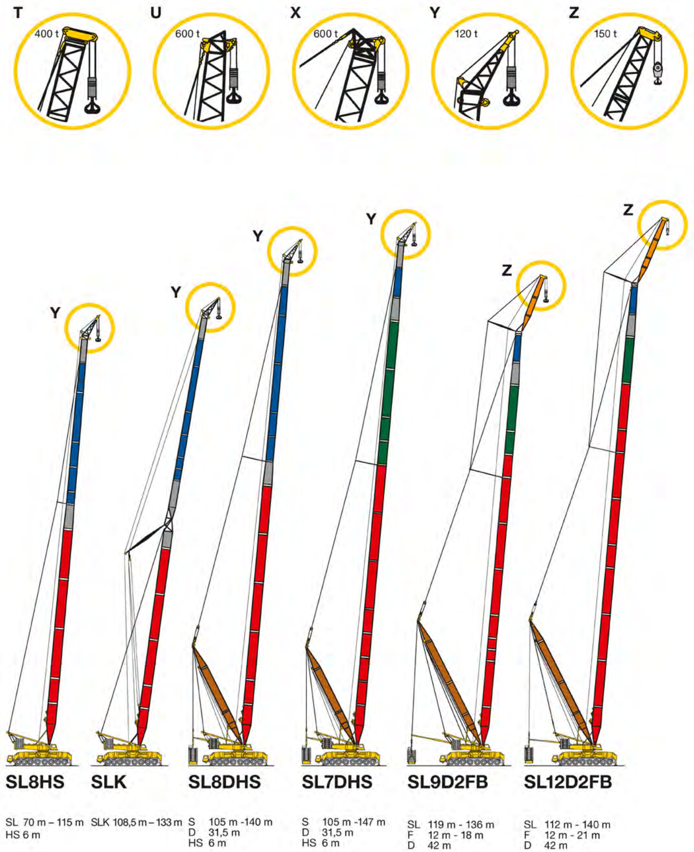
Figure 6: The wind kits (jib parts Y and Z) of a typical 750 ton lattice boom crane.
