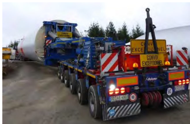
Figure 26: Tower transport using “clamps”
