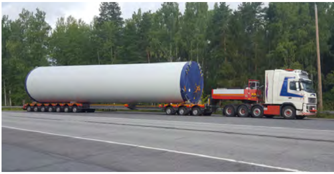
Figure 33: 4-axle tractor with 3-7 extendible semi lowloader loaded with tower section
