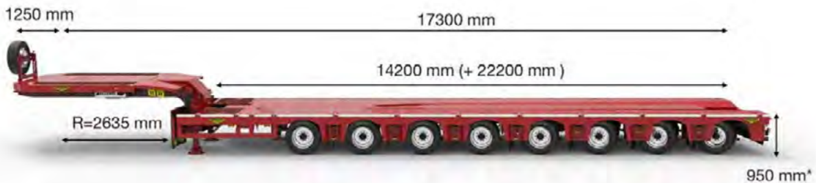
8 axle extendible semi lowloader
