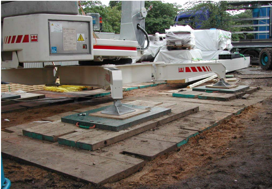
Correct Packing Under Outriggers (See 5.3)
