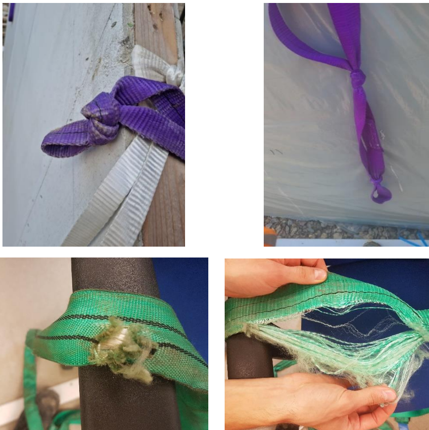
Figure 1 – Example of loads arriving on site with knotted and damaged lifting slings
