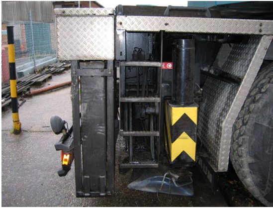
Fig. 1. Additional Access Ladders
