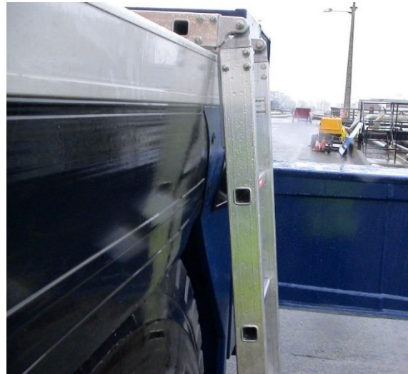
Fig. 4. Original Ladder Hanging Freely
