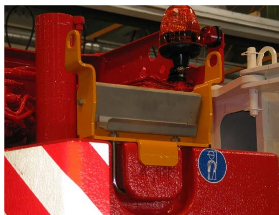
Automatic Ladder Latch with Anchor Point
