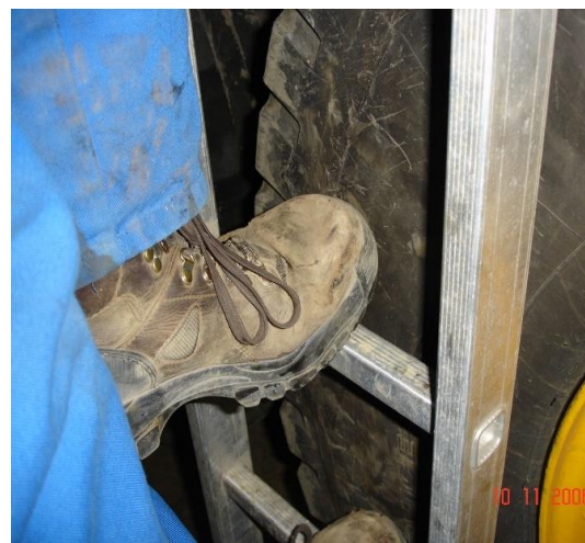
Fig. 2. Insufficient Foot Penetration
