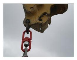
**Figure 12. –** Swivel allows unrestricted rotation but reduces available headroom
