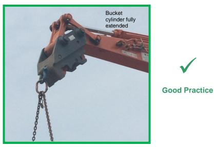
Figure 13. – Chain and master link can hang freely without obstruction
