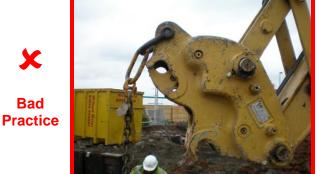
**Figure 15.** – Hitch tilted backwards with master link subject to twisting
