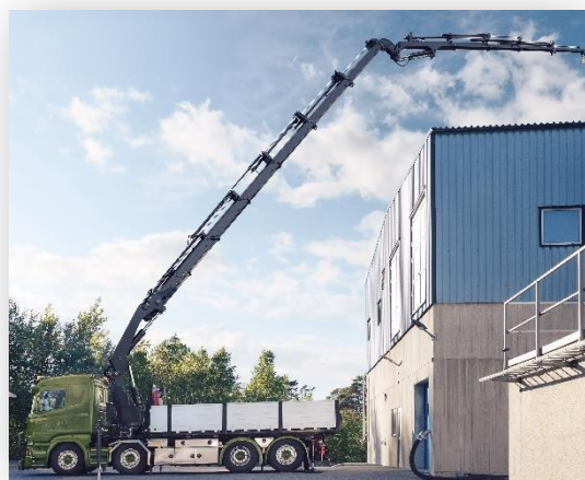
Figure 2: Lorry Loader Crane
