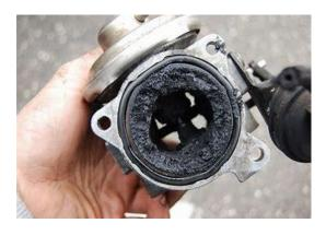
**Blocked Exhaust Gas Recirculation Valve**
