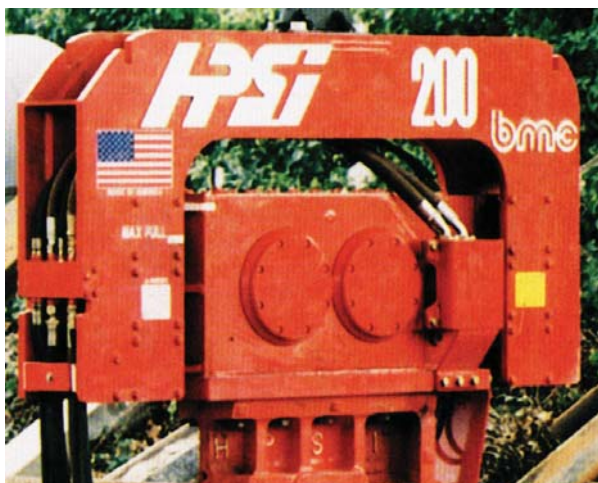
Figure 3.19 HPSI Model 200 Driving Sheet Piling
