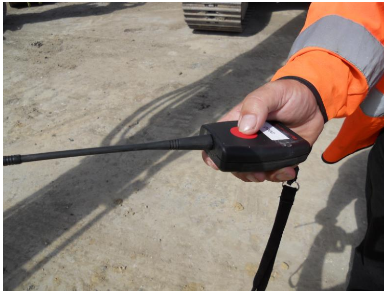
Figure F.5 - Handheld Remote Cut-off
