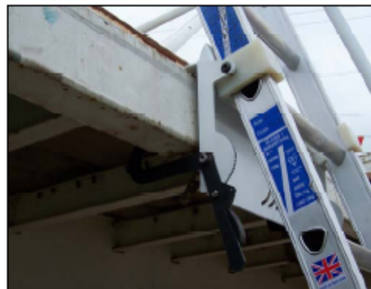
Figure 2 Showing ratchet clamping system
