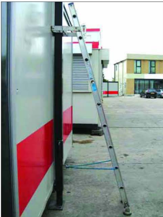
Figure 4 Specially designed ladder, fitted onto the cabin.
